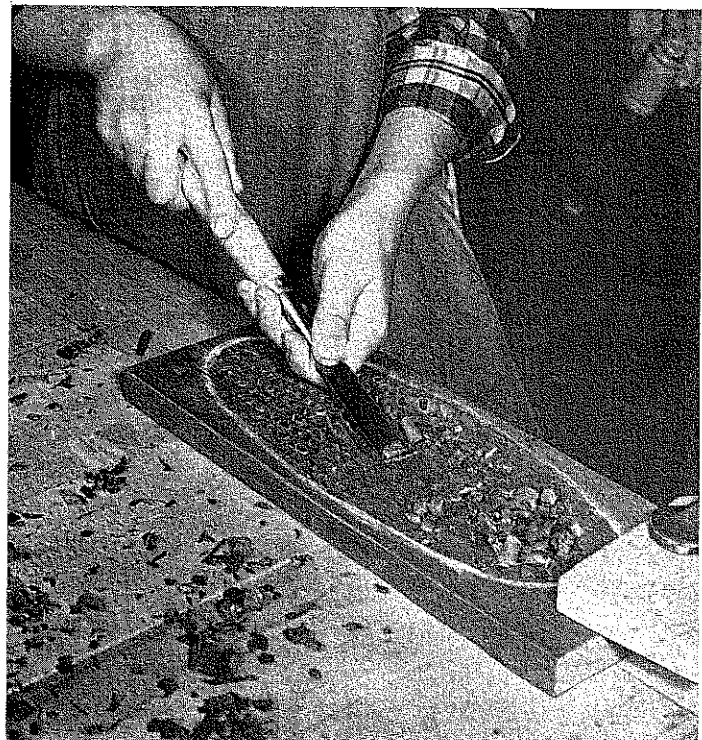
Fig. 3-3. Always cut away from your body when using edge tools.
