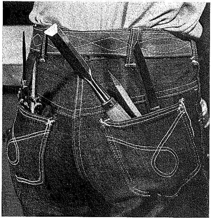
Fig. 3-2. Do not carry tools in your pockets—especially sharp-pointed tools.
