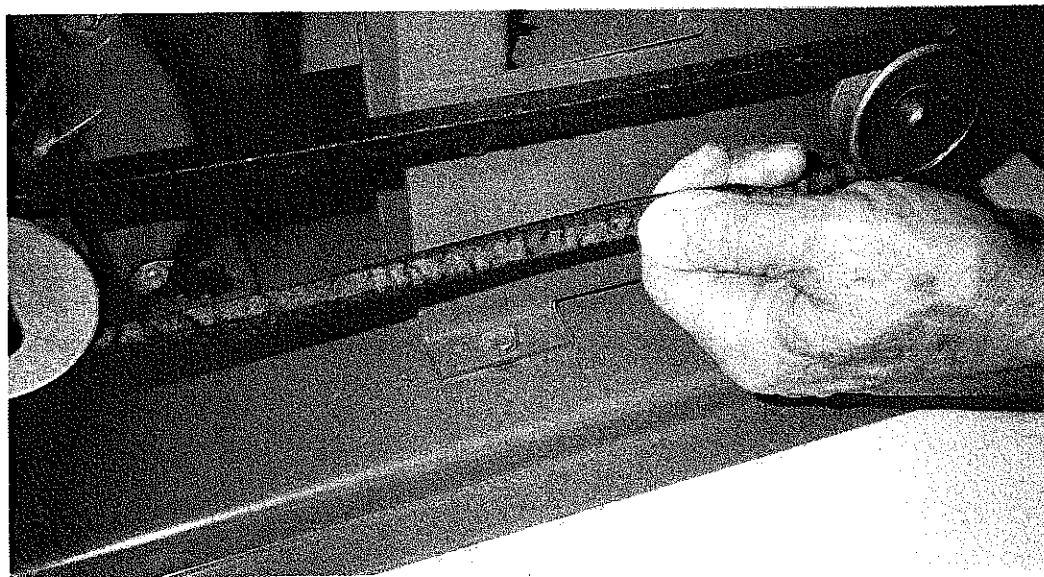
Fig. 3-5. A cracked and split drive belt is a sign of age. Replace the belt immediately.
